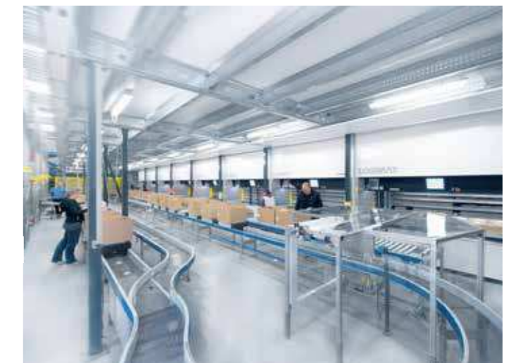
Several LOGIMATs can be used for the picking and storage of items, allowing other warehouse areas to be connected.
